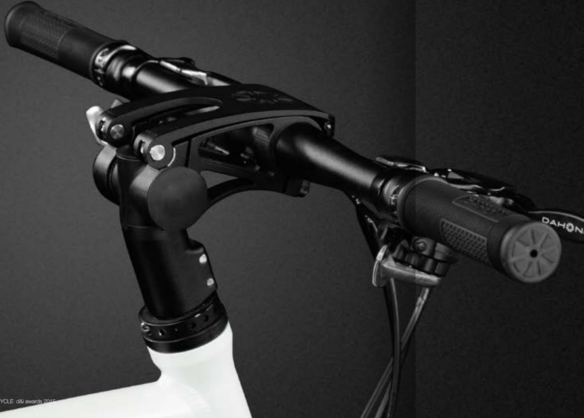
4D Quickpark Stem Paired with one of DAHON's patented folding pedal designs, you get a sturdy bike that goes from 3-D to 2-D in seconds, and stores almost completely flat.
