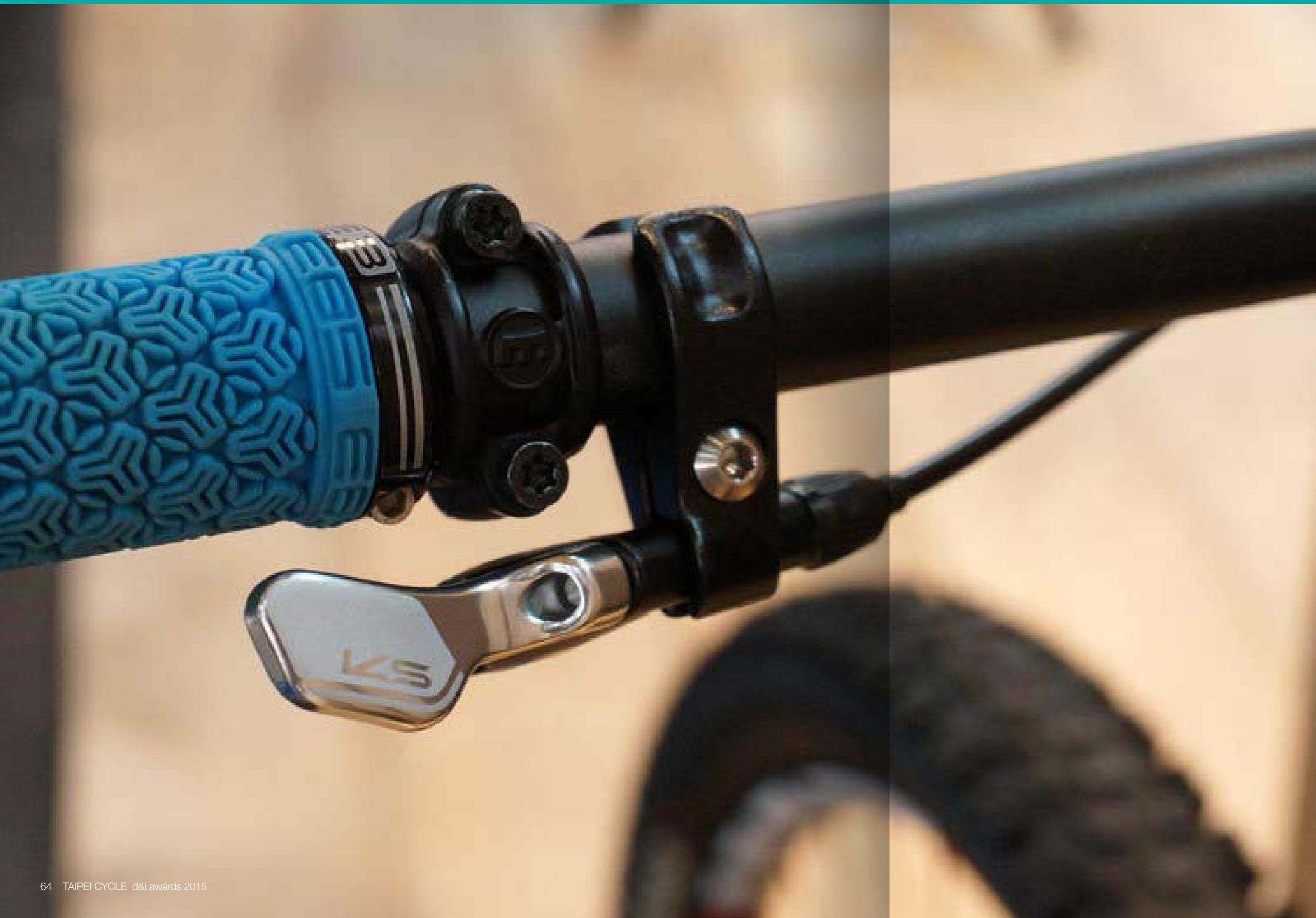
It's a simple little thing, but then again the world was turned upside down when shifters went down under. With the advent of 1x drivetrains, we saw a vacancy downstairs just begging for a hot neighbor to move in: the SOUTHPAW underbar remote specifically designed for bikes with 1x drivetrains. Sold as an accessory only, SOUTHPAW uses an innovative split clamp, allowing for 4-axis adjustment for perfect ergonomics and feel.
