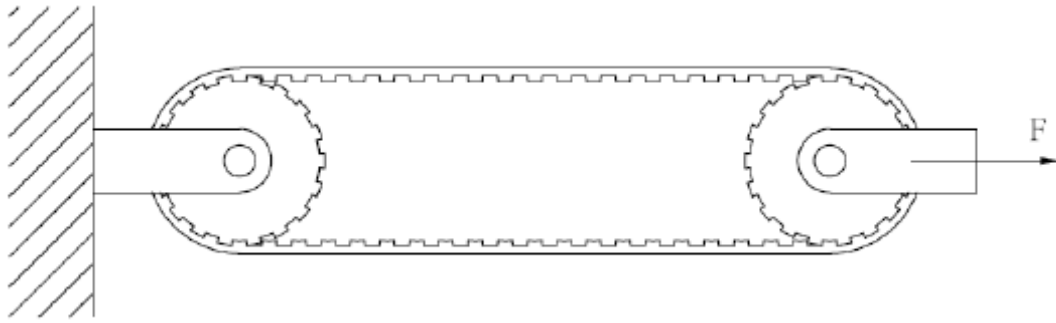
Figure 5 — Drive belt — Tensile strength test
