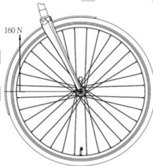
Figure 35 — Front mudguard: tangential obstruction test
